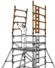
**7** Add two more diagonal braces between the 5th and 7th rungs. If finishing at this height (4.2m platform) reposition the fixed deck to the 8th rung on the tower. Fit a trapdoor deck alongside it, with the hinges towards the outside of the tower, and the trapdoor next to the ladder. Add a single diagonal between the 7th and 9th rungs as shown. Climb up the ladder, and from the protected trapdoor position, fit the guardrails on the 9th and 10th rungs, in that order, on both sides of the tower.
